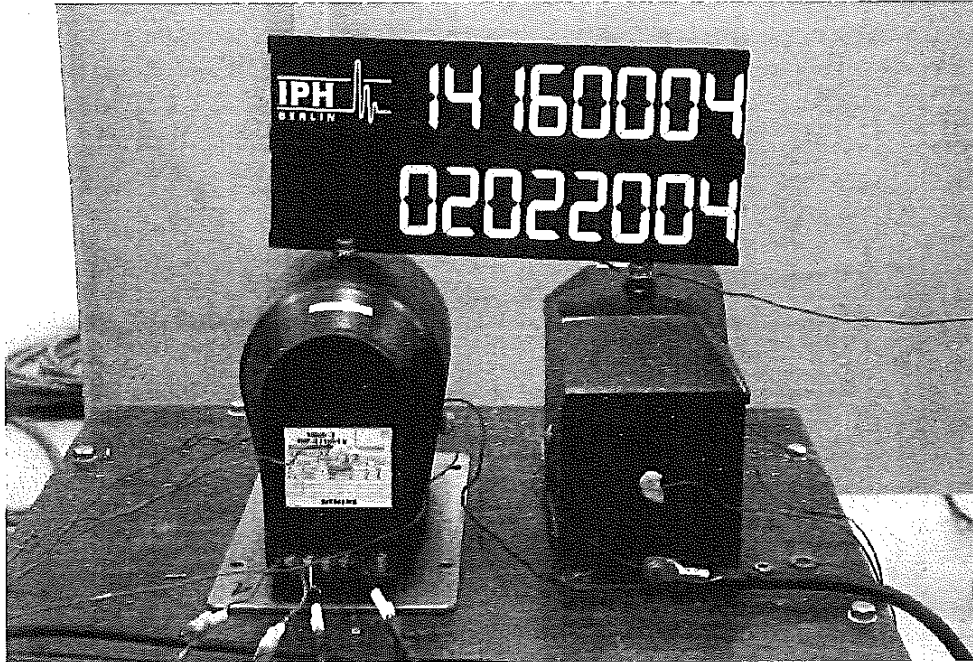
Figure 7: Test object during the temperature-rise test (right sample)
